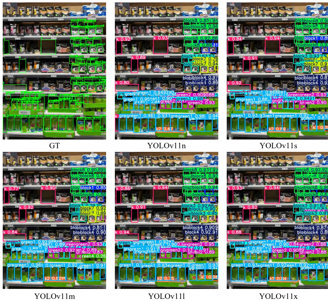
Figure 5 Comparison of Per-Category Product Predictions for Different Models Using the Same Shelf Image
