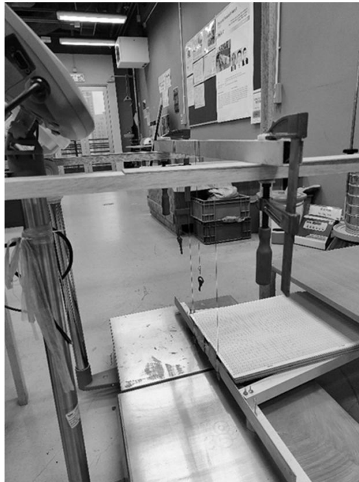
Figure 10 Align the Reference Beam with the Survey Plate by a Pair of Strings
