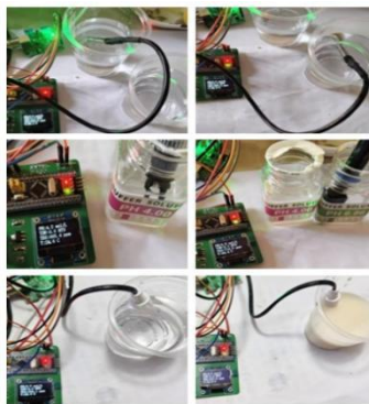
Figure 9 Temperature, pH and TDS Sensor Performance Test Process
