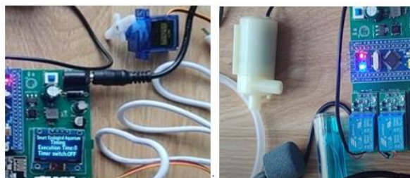
Figure 10 Performance Test of Servo and Water Pump Actuator
