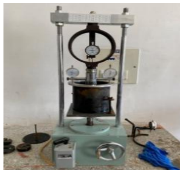
Figure 3 CBR Test under Loading
