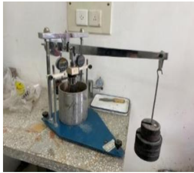
Figure 4 Resilient Modulus Test in Progress
