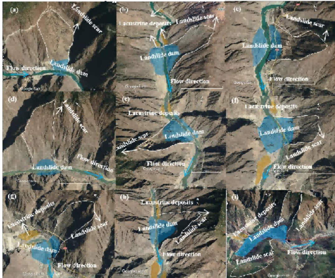
Figure 4 Nine Damming Landslides in the Upper Reaches of Jinsha River. (a) Lawa Landslide; (b) Temi Landslide; (c) Niuying Landslide; (d) Xiawagui Landslide; (e) Xuelongnang Landslide; (f) Suoduoxi Landslide; (g) Suwalong Landslide; (h) Biji Landslide; (i) Wangdalong Landslide. Image Credit: Google Earth
