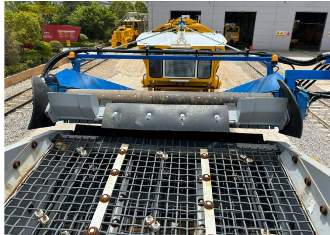
Figure 4 Double-Layer Feeding and Material Distribution Mechanism
